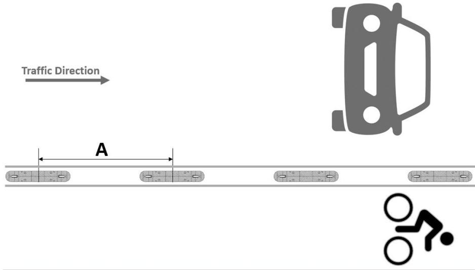
The parallel positioning of TreeTop Premium Rubber Bike Lane Delineators is most suitable when there's limited available buffer zones (i.e.; painted lines). To ensure optimal safety, it is recommended to maintain a spacing between centers (A) of 6ft between the delineators, while not exceeding 8ft.
