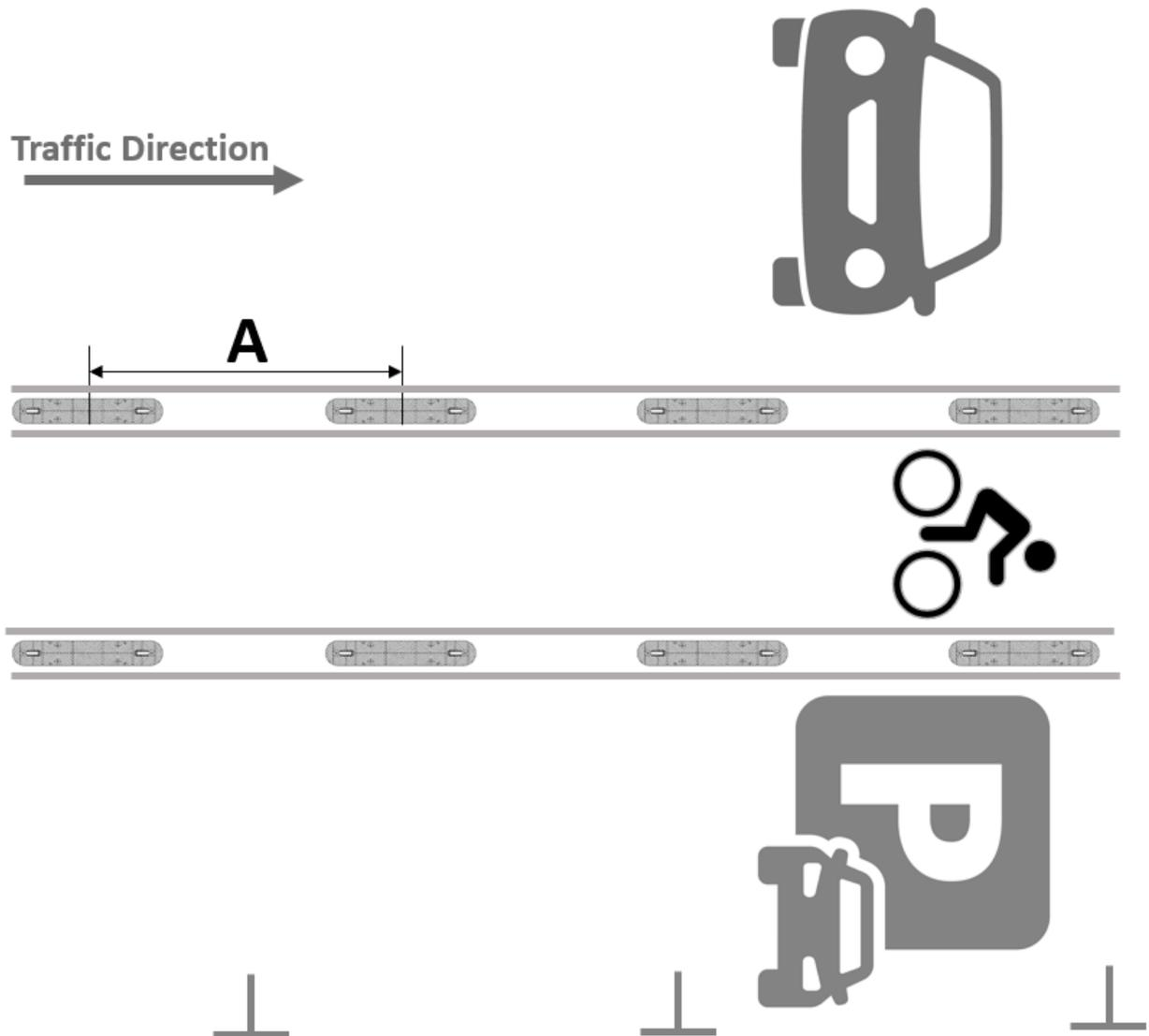
The 3" High Crossover Premium Rubber Bike Lane Delineator is designed to slow down vehicles to 1-2 mph and allow vehicles to crossover slowly and safely into roadside parking spaces or right-turn lanes. For applications that do not require vehicles crossing over, check out Treetop's 5" High Curb Premium Rubber Bike Lane Delineators.
