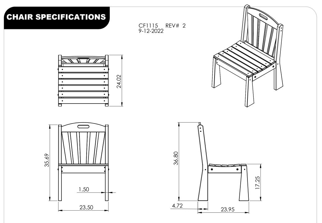
CONSTRUCTION MATERIALS: Recycled Plastic HARDWARE: Stainless Steel
