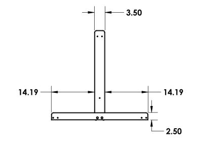
CONSTRUCTION MATERIALS: Recycled Plastic HARDWARE: Stainless Steel
