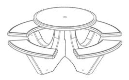
**Caution:** Table needs to be assembled on a level, hard or compacted surface in its final location. Once table is assembled it should not be moved fully assembled as structural damage may result. Failure to follow these guidelines may cause undo stress on table components and cause structural failure.
