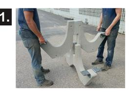
Attach eight seat brackets (#6) to leg (#5) to top and bottom interlocking leg with (#8) 3/8" x 5 1/2" hex Bolts, (#9) 3/8" locking hex nuts, and (#11) 3/8" flat washers. Note: use 3/8" flat washers on both sides of bracket. After installation of brackets on interlock legs, use brackets for lifting and assembly of Interlock legs.
