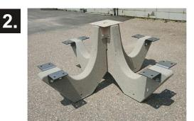
Attach (#2) table to leg bracket to assembled interlock base utilizing (#8) 3/8" x 5 1 /2" hex bolts, (#9) 3/8" locking hex nuts, (#10) neoprene pads for each bench bracket, and (#11) 3/8" flat washers. Note: use 3/8" flat washers on both sides of bracket.
