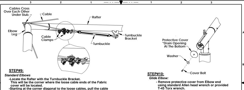
and Fabric corner hole over the stub welded to the tip of the Elbow. Cable must go over first.
