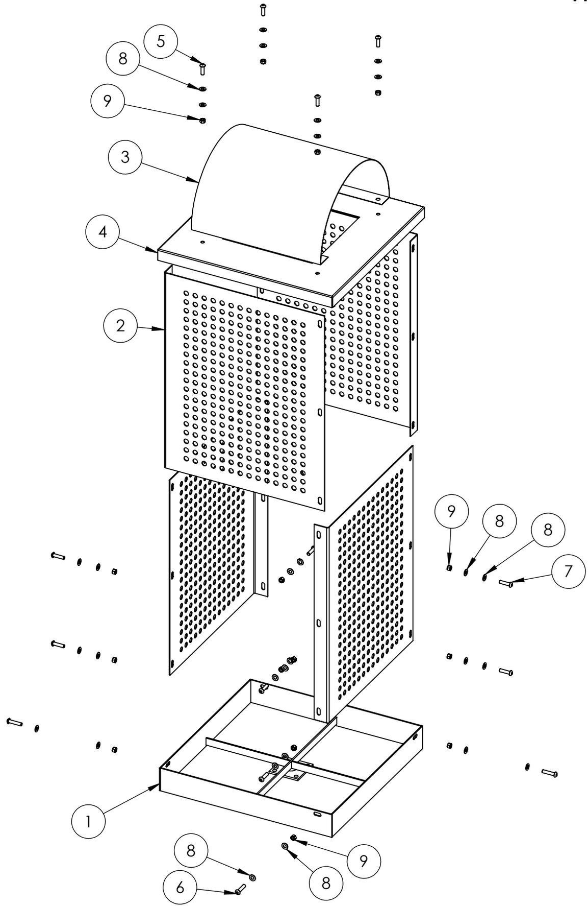
1. With a 7/16" drill bit, drill out the holes of the side panels, arch, lid, and base.
