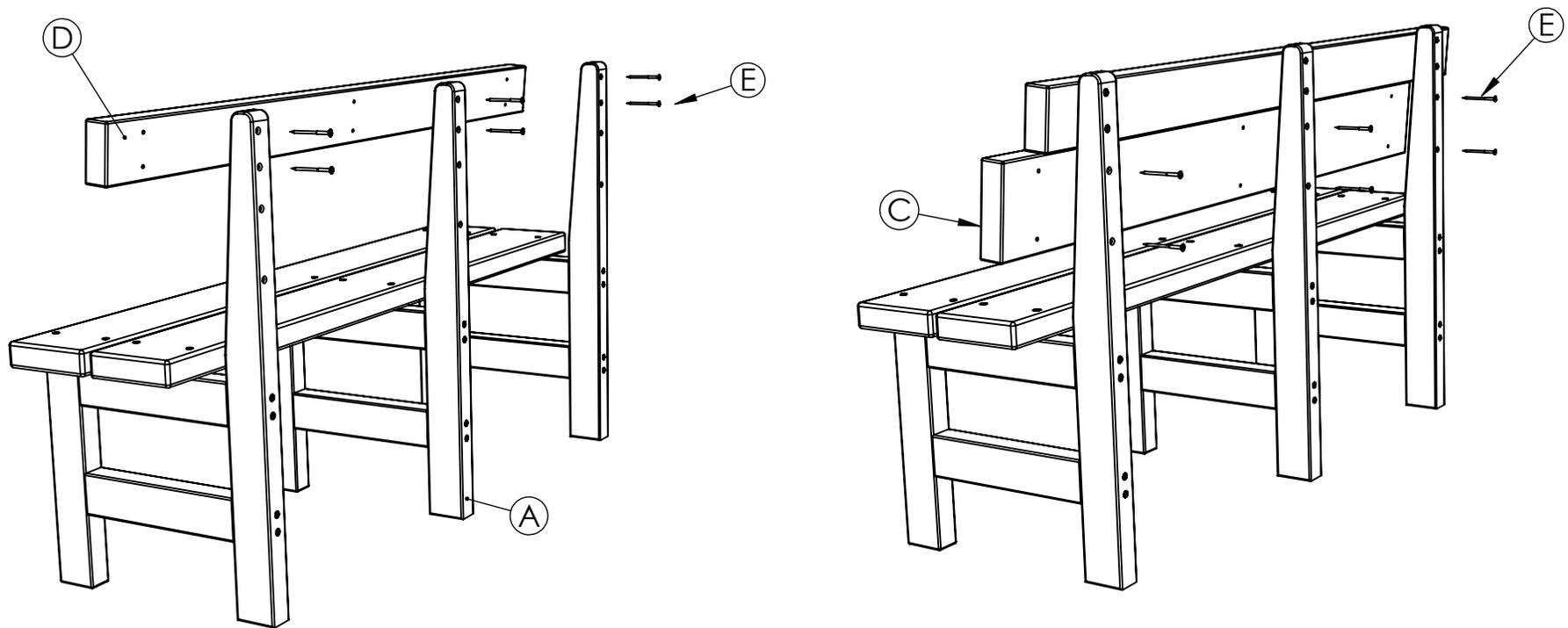
**NOTE: IT IS IMPORTANT TO NOT OVER TIGHTEN THE SCREWS GOING INTO THE BACK BOARDS OR THE SCREW WILL PROTRUDE OUT INTO THE FRONT OF THE BOARDS**
