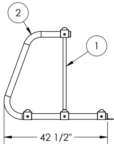
1. Drill plastic out of the mounting holes on the ends, rails and fence using a 7/16" dia. drill bit.
