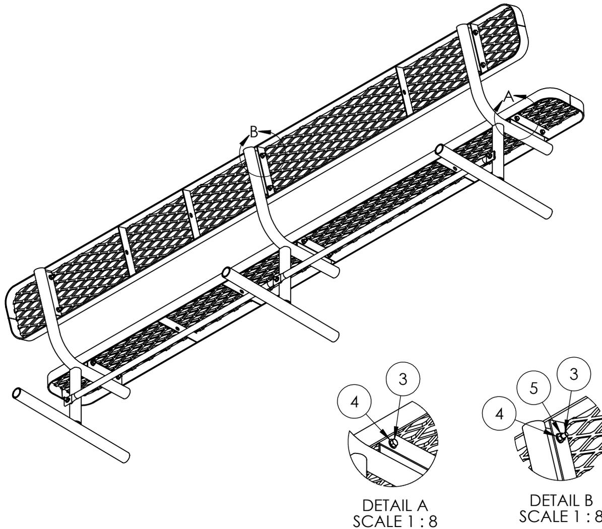
1. Drill plastic out of the mounting holes on the seat, back and stands using a 7/16" diameter drill bit.
