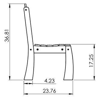
CONSTRUCTION MATERIALS: Recycled Plastic HARDWARE: Stainless Steel
