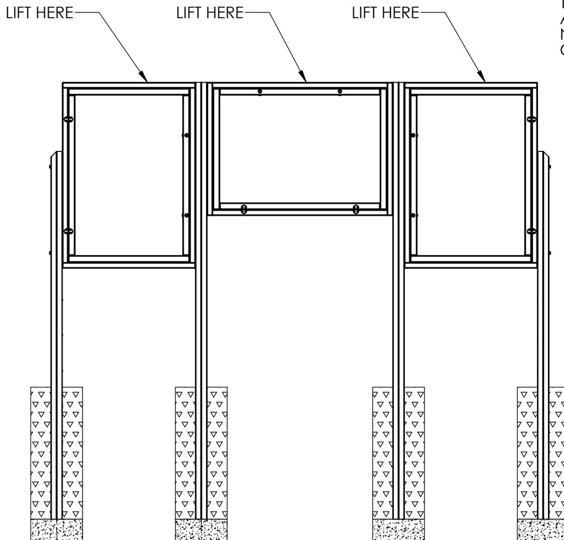
WITH HELP FROM OTHER PEOPLE, CAREFULLY TILT MESSAGE CENTER ASSEMBLY INTO HOLES AND BRACE MESSAGE CENTER. LEVEL AS NECESSARY AND FILL HOLES WITH READ-TO-MIX CONCRETE. ALLOW TO DRY AND REMOVE BRACING.
