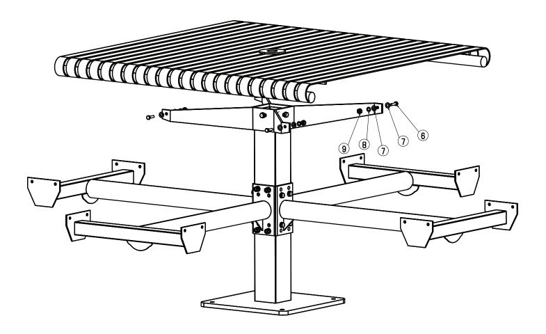
Attach the square table top to the table support bracket using the specified hardware.
