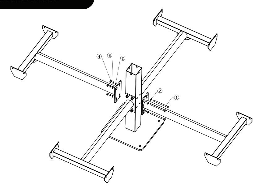
Attach the side frames to the pedestal frame using the specified hardware.
