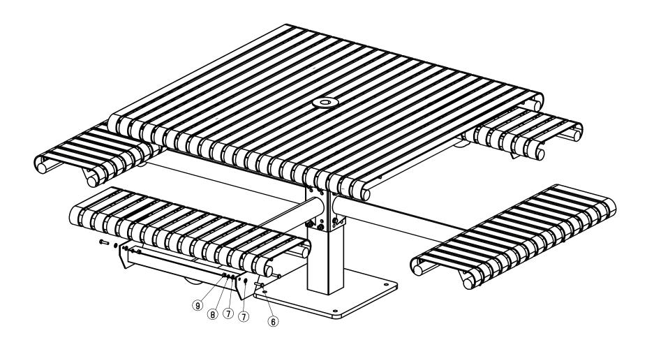
Attached the seat tops to the side frames using the specified hardware. Fully tighten all hardware with appropriate wrenches.
