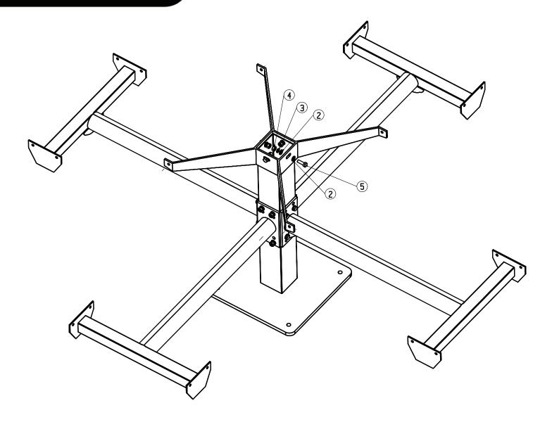
Attach the table support bracket to the pedestal frame using the specified hardware.
