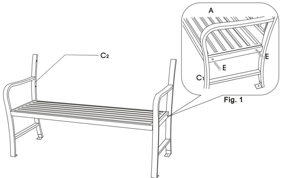
**Step # 2:** Attach the Backrest (B) to the Left Armrest (C2) and Right Armrest (C1) by using Bolts (D). **Hand tighten!** Adjust the bench to a level position and tighten all the Bolts with Allen Wrench (F) (Provided).
