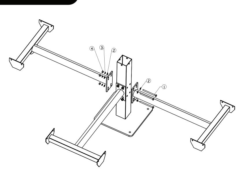
Attach the side frames to the pedestal frame using the specified hardware.
