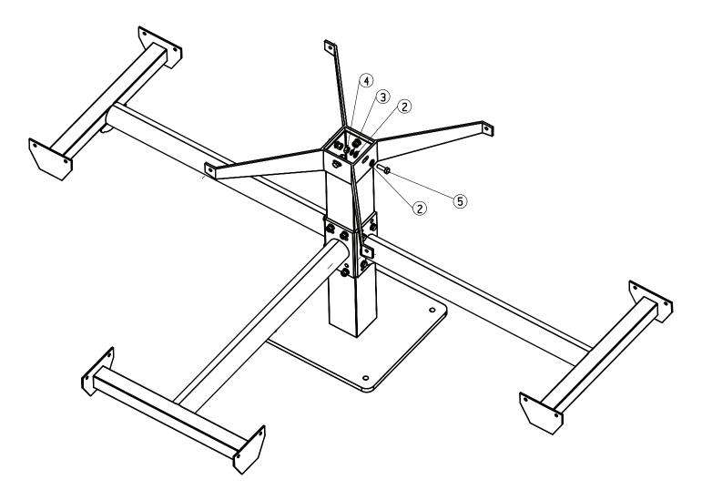
Attach the table support bracket to the pedestal frame using the specified hardware.
