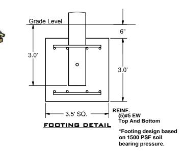
These drawings are for reference only and should not be used as construction details. Materials, fasteners, and foundations are subject to change if professionally sealed engineering drawings are required. Designed for 93 MPH Basic Wind Speed.
