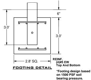
These drawings are for reference only and should not be used as construction details. Materials, fasteners, and foundations are subject to change if professionally sealed engineering drawings are required. Designed for 93 MPH Basic Wind Speed.
