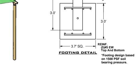
These drawings are for reference only and should not be used as construction details. Materials, fasteners, and foundations are subject to change if professionally sealed engineering drawings are required. Designed for 93 MPH Basic Wind Speed.
