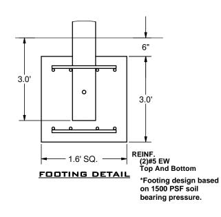
These drawings are for reference only and should not be used as construction details. Materials, fasteners, and foundations are subject to change if professionally sealed engineering drawings are required. Designed for 93 MPH Basic Wind Speed.
