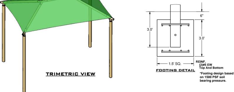
These drawings are for reference only and should not be used as construction details. Materials, fasteners, and foundations are subject to change if professionally sealed engineering drawings are required. Designed for 93 MPH Basic Wind Speed.
