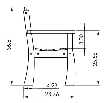
CONSTRUCTION MATERIALS: Recycled Plastic HARDWARE: Stainless Steel
