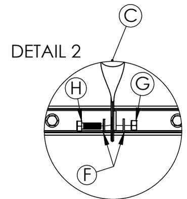
Angle support brace connection to center channel
